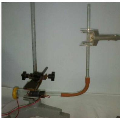
Fig. 12. Experimental setup for determining quantitative parameters of substance transfer in meat under the influence of electric current
