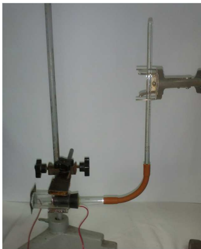
Fig. 19. Experimental setup for determining the quantitative parameters of substance transfer in meat under the influence of heat flow and electric current
