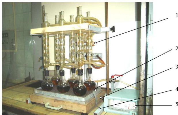
Fig. 53. General view of the hydrolysis unit: 1 – water condenser; 2 – flask with hydrolysate; 3 – sand bath; 4 – heating surface; 5 – MP-64-02 temperature controller
